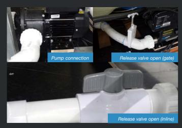
Check pump connection and release valves
